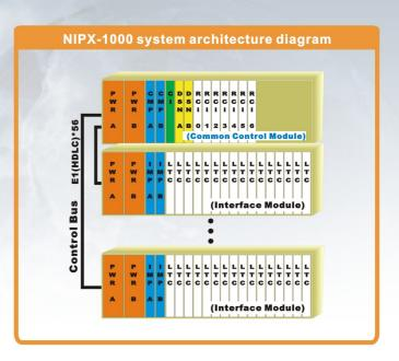
The most efficiency design with large capacity which constructed in 23" standard shelf, each shelf support 256 free ports and easily expand to 512 ports by stack 2 shelves, this is model called NIPX1000S. when the configuration exceed 512 ports, a common control module can be equipped for expansion up to 7168 ports which handle 28 shelf as well, this is model called NIPX-1000.
